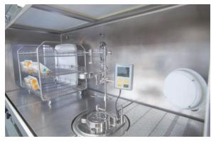
The Barrier Isolators type **VHPIT** are designed in order to grant the sterile handling and transfer of products throughout the Process Equipments.
