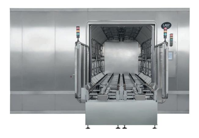
The Sterilizers type **TS-AS** & **TS-OW** are specifically designed for the Terminal Sterilization of liquids contained in sealed containers (plastic bags, glass bottles, BFS bottles, syringes, ampoules, etc.) as they are prepared to provide an automatic differential pressure compensation based on product probes (RTD) temperature measurement ( $\Delta$ T). This kind of control prevent the deformation, damaging and bad coloring of the plastic containers.
