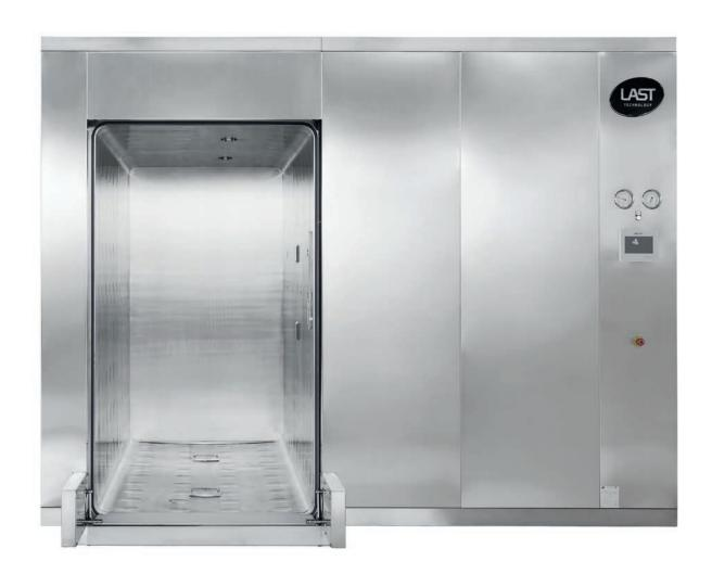
The Sterilizers type **ETO** are designed for the sterilization by Ethylene Oxide of heat sensitive products such as plastic syringes, perfusion sets, dialysis cartridges, heat sensitive rubber products and special surgical instruments.
